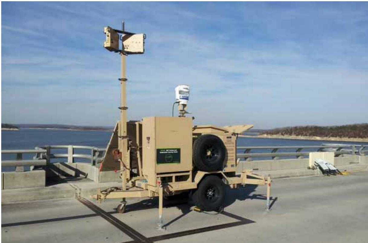
**Figure 1 - Blighter coastal security radar mounted on trailer-based mobile surveillance platform (Deployed at the Truman Dam, MO, USA)**
