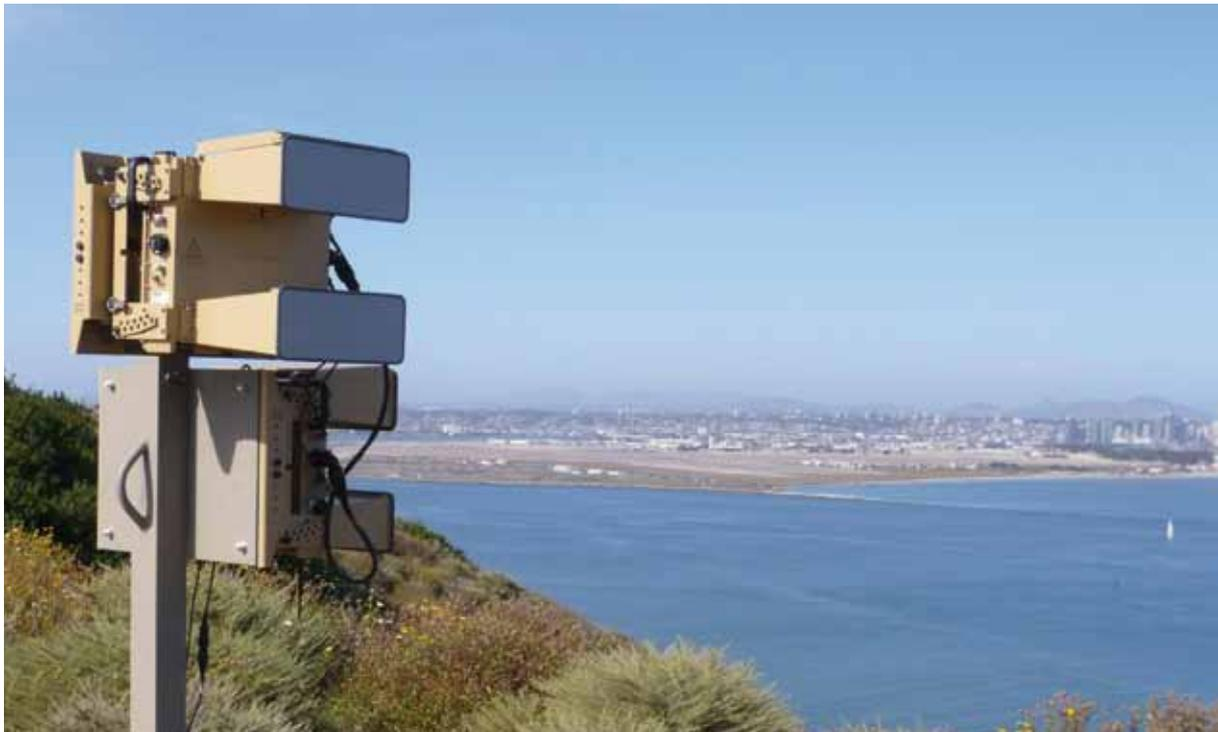
**Figure 4 - Blighter C400 series coastal security radar (Point Loma, San Diego, CA, USA)**
