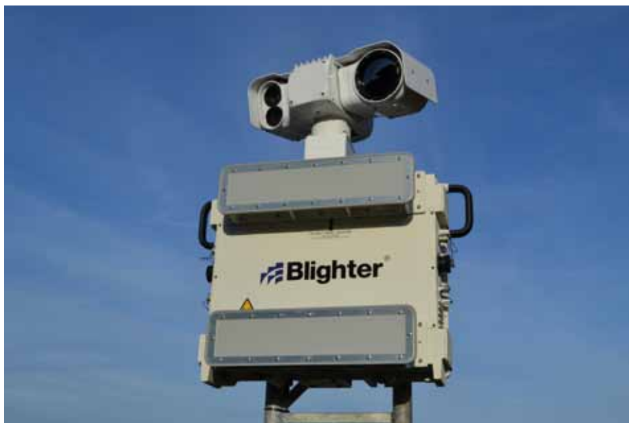
Figure 3 - 90 degree e-scan radar with co-mounted thermal camera system
