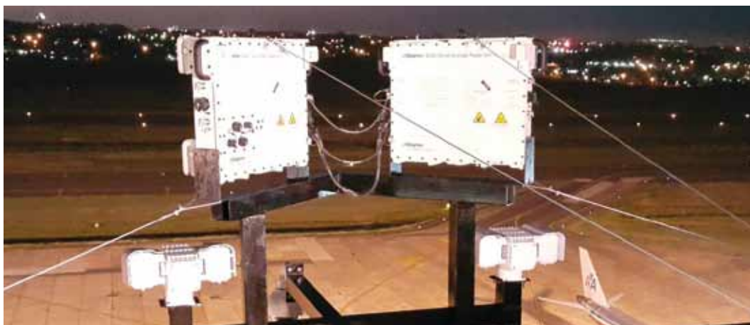
Figure 2 - Typical installation of 180 degree e-scan Doppler radar at a large international airport in South America
