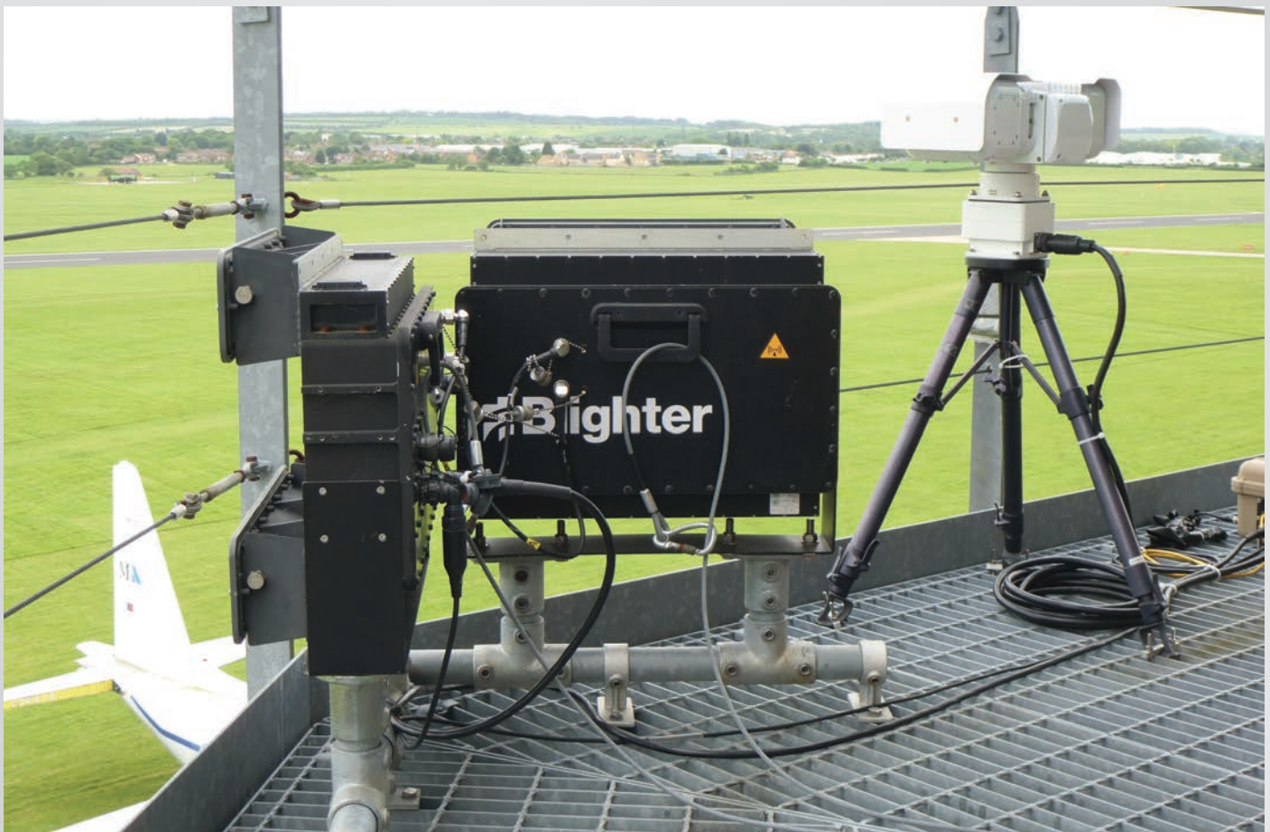
Blighter B422 E-scan Radar and Liteye Aquila Daytime and Thermal Camera System at Airport
